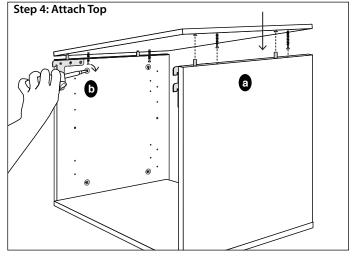
(a) Attach Sides to Bottom. (b) Lock Cam by turning clockwise until snug.
